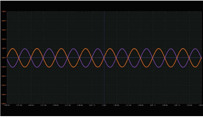
Figure 6. Waveforms of a variable gain inverting amplifier using a potentiometer.
